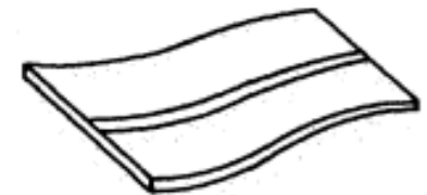
(f) BUCKLING DISTORTION
